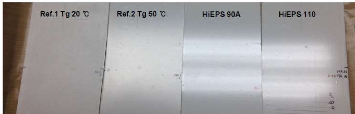
<White top coat samples after 20 days humidity acceleration test>
